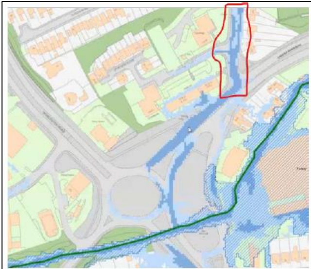
Figure 12: Surface water modelling undertaken in support of the planning process for Hoo Brook Roundabout in Kidderminster
